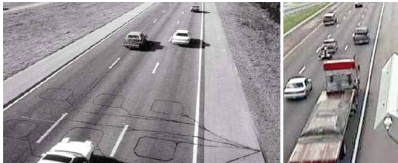
Figure E: Field deployed inductive loop (left) and roadside acoustic sensor (right) (FHWA, 2003)
